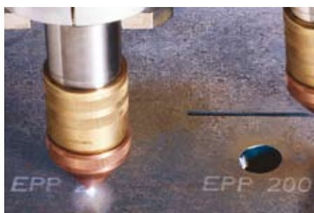
Plasma cutting and marking with the same torch
