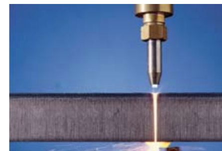
Oxyfuel cutting up to 200 mm material thickness
