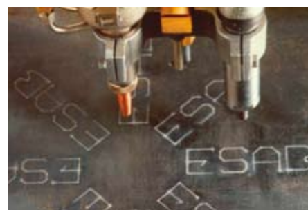
Left: Powder marking right: Compressed air marking
